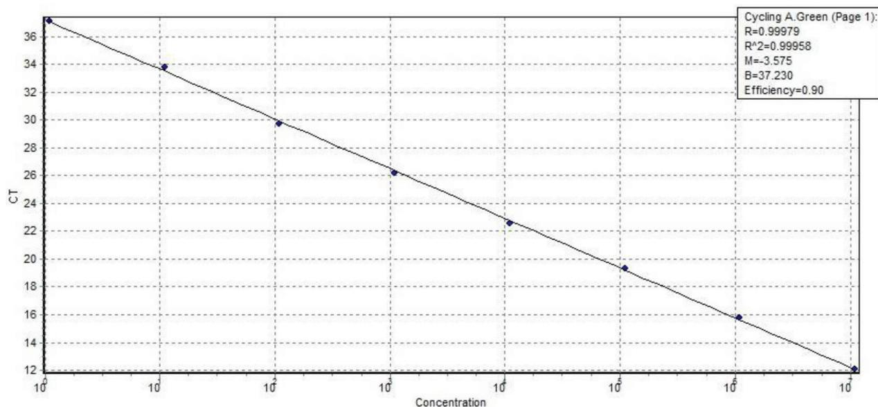
**Figure 3.** Linearity of the standard curve, the detection limit of the assay was 12 copies/reaction with a corresponding  $C_T$  value of 36.79.
