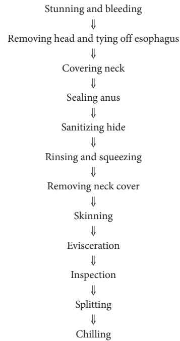
Figure. Flow diagram of pre-evisceration, skin-on carcass sanitation of beef carcasses.
