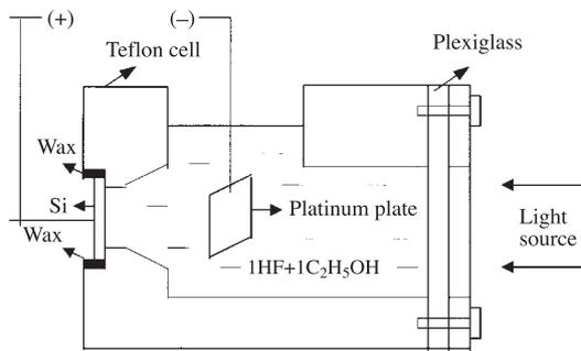
**Figure 1.** Electrochemical set up
