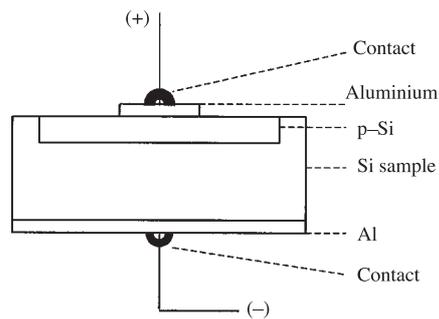
**Figure 2.** Configuration for the electrical measurements.
