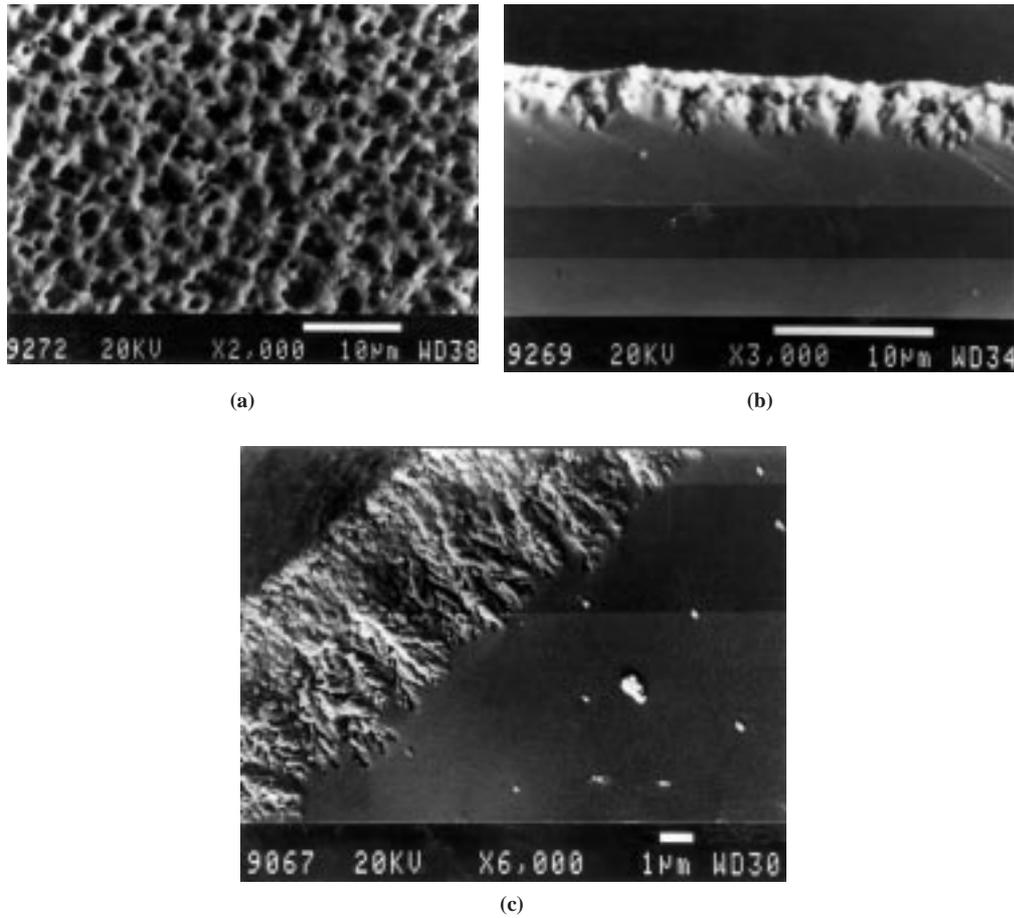
**Figure 4.** p-Si structure obtained at high current density ( $30\ \text{mA}/\text{cm}^2$ ). a) surface film, b) cross-section film, c) cross-section film for 30 min.
