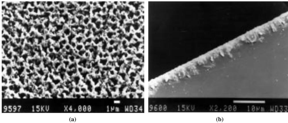
**Figure 3.** p-Si structure obtained at low current density (5 mA/cm<sup>2</sup>). a) surface film, b) cross-section film
