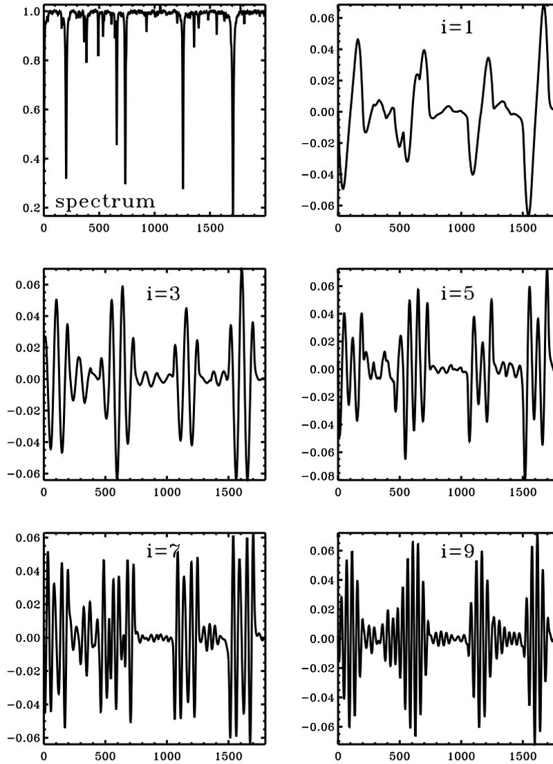
**Figure 6.** The SVD process involves decomposition of the original spectra into basis vectors which are stored in columns of the matrix  $\widehat{Des}$ . The same sharp-line spectrum as in the previous graphs is shown here in the upper left panel together with five typical basis vectors (every second one, as indicated).
