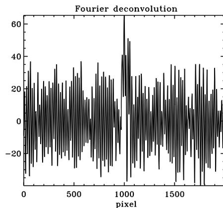
**Figure 5.** A rather typical case of the Fourier de-convolution. We know that the BF differs from zero over a small interval of some 100 – 200 pixels, yet it is determined over the whole span of the original spectra. In addition, small errors in the sharp-line spectra frequently become amplified in the Fourier-transform division stage. This results in strong fringing of one or several spatial frequencies invalidating the whole process.
