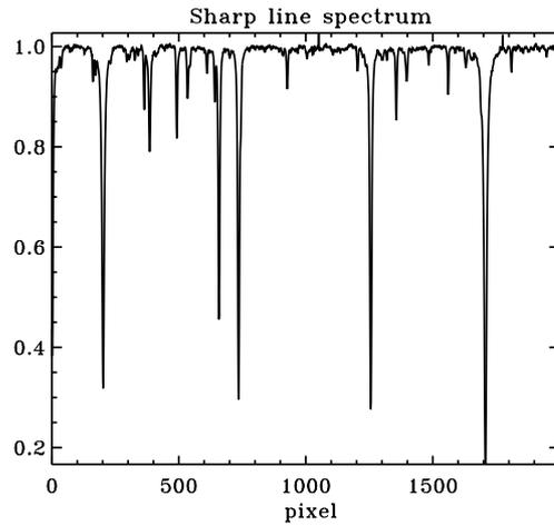
**Figure 2.** A typical case of a high resolution spectrum of high quality. Such spectra must be re-binned to equal velocity spacing, but – for practical purposes – one uses spectra as one-dimensional functions or vectors defined over a certain number of pixels. Typical spectra have now lengths of 1000 to 4000 pixels.
