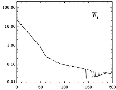
**Figure 8.** Elements of the diagonal array  $W$  for the SVD of the sharp-line spectrum in Figure 2. The solution of the BF determination process that we propose involves use of only a few first elements of this array. This corresponds to discarding of a large amount of basis vectors so that the BF shapes are represented with some loss of resolution. The next figure shows the BF determinations based on only the first 5, 10, 20 or 30 singular values.
