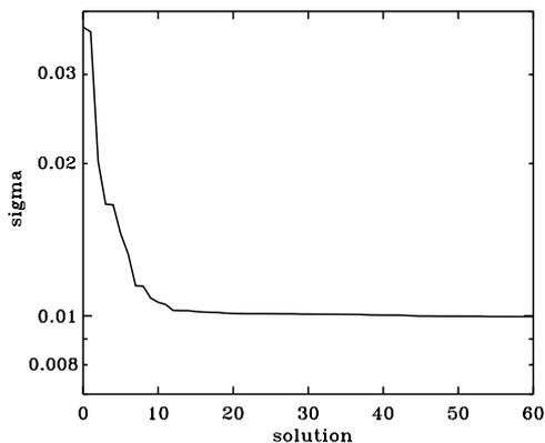
**Figure 11.** The answer to the question posed in the caption to Figure 10 is in the plot of the quality of fit. For  $k \simeq 12 - 15$  the standard error of the fit stops decreasing and this is the place to fix the number of the singular values. Addition of more singular values does increase the resolution, but one then models the noise in the broadened spectrum. In this case the  $S/N$  was 100 and the asymptotic error level is indeed 0.01.
