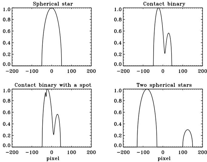
**Figure 1.** Four schematic examples of broadening functions. The first case (upper left) is the case of a single star rotating uniformly. The case of a contact binary (upper right) illustrates how the shape of the binary is projected into the velocity space. For two detached stars (lower right) the two peaks are disjoint but we still can define a single BF. The star spots correspond to missing flux at certain velocities. Their manifestation would be indentations in the BF (lower left).
