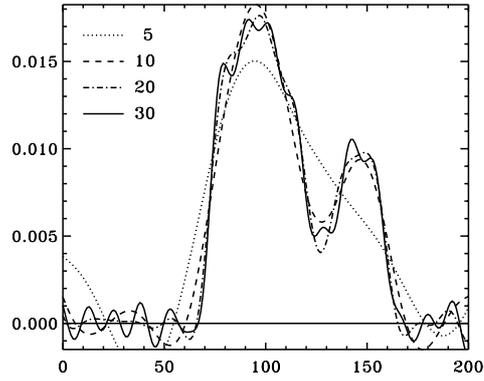
**Figure 9.** The BF (the same as the dotted line in Figure 3) restored through the SVD process from the broadened spectrum (as in the lower panel of Figure 3, but with an added noise at  $S/N = 100$ ). The power of the SVD is demonstrated by the fact that as few as 10 or 20 first singular values are sufficient for an excellent determination, which is much superior to the cross-correlation function (compare this figure with Figure 4).
