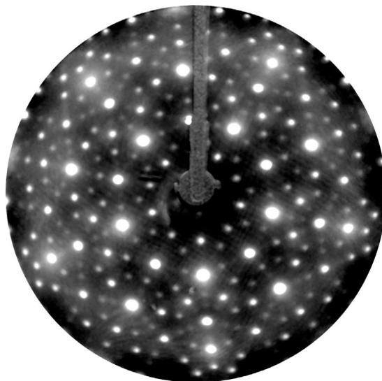
**Figure 1.** Diffraction pattern from a prepared pentagonal surface of Al-Pd-Mn quasicrystal. The electron energy is 120 eV. The immense number of spots with decreasing intensity is a measure of the size of surface region with correlated scatterers in which the quasicrystalline perfection prevails.
