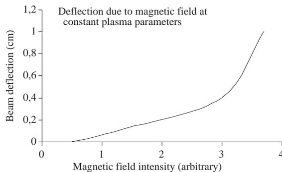
**Figure 5.** Deflection of the electron beam under the influence of a magnet with arbitrary field intensity, as the magnet approaches the discharge tube.
