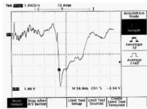
**Figure 3.** Typical current variation of the electron beam.
