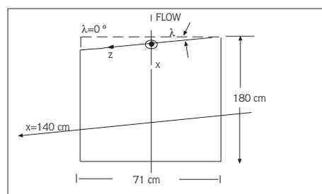
Figure 1 Top view of the test plate
