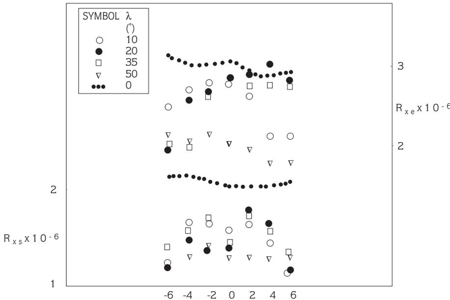
Figure 2. Spanwise variation of  $R_{xs}$  and  $R_{xe}$  at  $x=140$  cm on swept plates.
