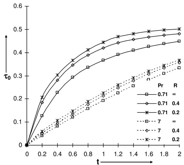
Figure 4. Skin-friction profiles at the plate  $y = 0$ .
