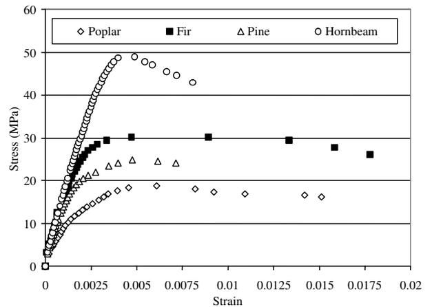
Figure 4. Compressive stress-strain curves of timber loaded parallel to the grain.
