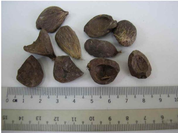
**Figure 3.** Various shapes of OPS aggregate.
