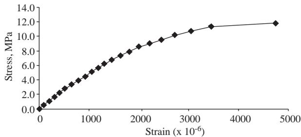
Figure 9. Stress-strain curve for OPS concrete.
