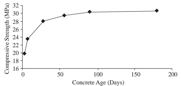
**Figure 6.** Compressive strength development of OPS concrete.
