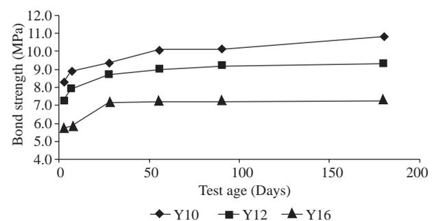
**Figure 8.** Bond strength development of OPS concrete.
