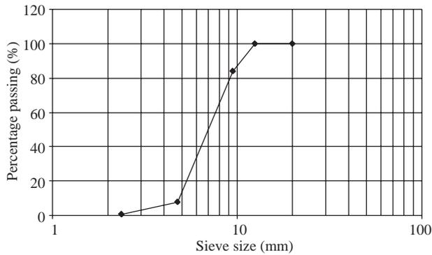
**Figure 4.** Particle size distribution of OPS aggregate.
