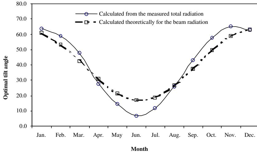
**Figure 5.** Monthly optimal tilt angles found theoretically for the beam radiation and those derived from the measured total radiation.
