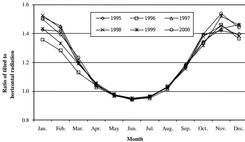
**Figure 2.** The ratio of tilted to horizontal solar radiation on a monthly basis for various years (the angle of the tilted surface is equal to the latitude of Ankara).
