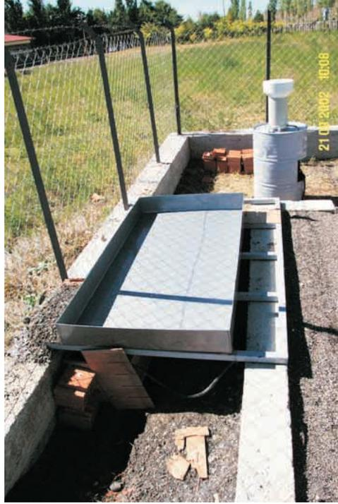
**Figure 3.** Snowmelt lysimeter and tipping bucket rain gauge at Güzelyayla Station. (Lysimeter 50 cm above the ground surface).
