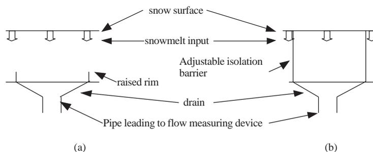
Figure 1. Snowmelt lysimeter configurations a) unenclosed b) enclosed.
