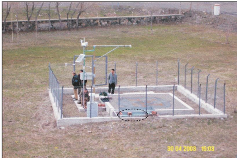
**Figure 2.** View of the Güzelyayla automatic snow pillow and automatic weather station. (Circle indicates the location of the snowmelt lysimeter).
