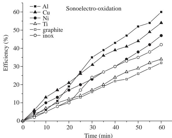
Figure 2. Cyanide degradation by sonoelectro-oxidation.
