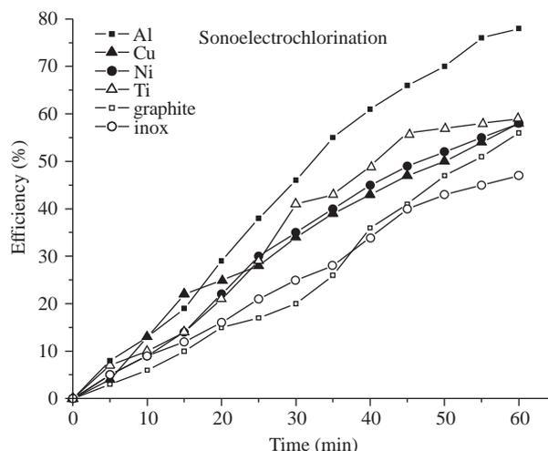
Figure 3. Cyanide degradation by sonoelectrochlorination.
