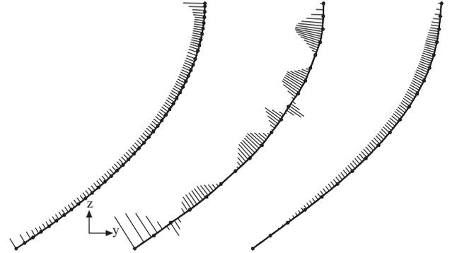
**Figure 2.** (a) Original, (b) distorted, (c) faired Wigley hull mid-section (1500 iterations, 95% of improvement in the objective function).
