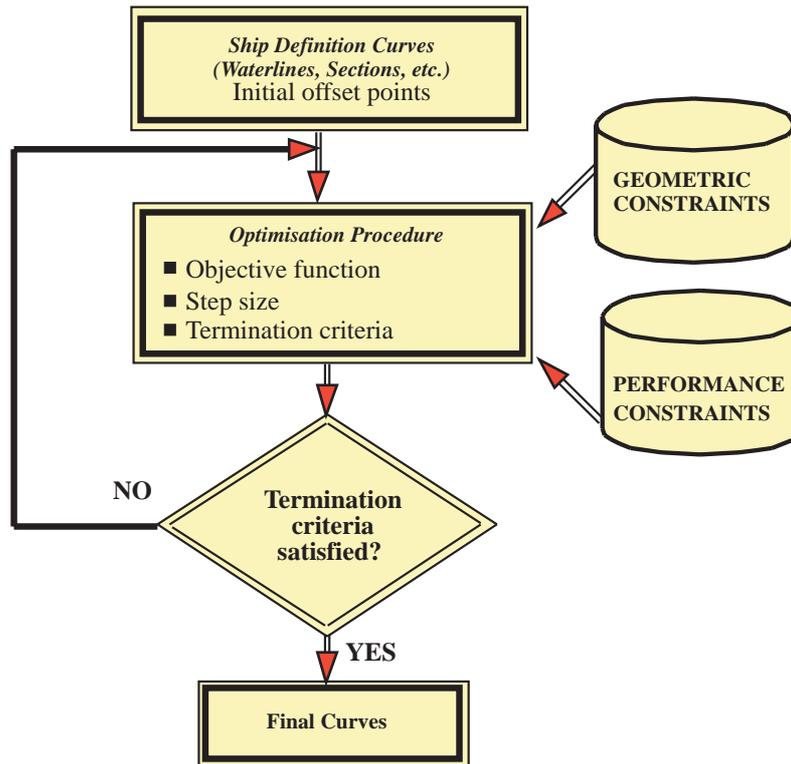
**Figure 1.** Structure of the optimisation based ship lines fairing procedure.
