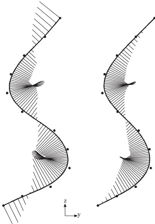
**Figure 3.** (a) Initial and (b) faired bulbous bow section (952 iterations, 45% of improvement in the objective function).
