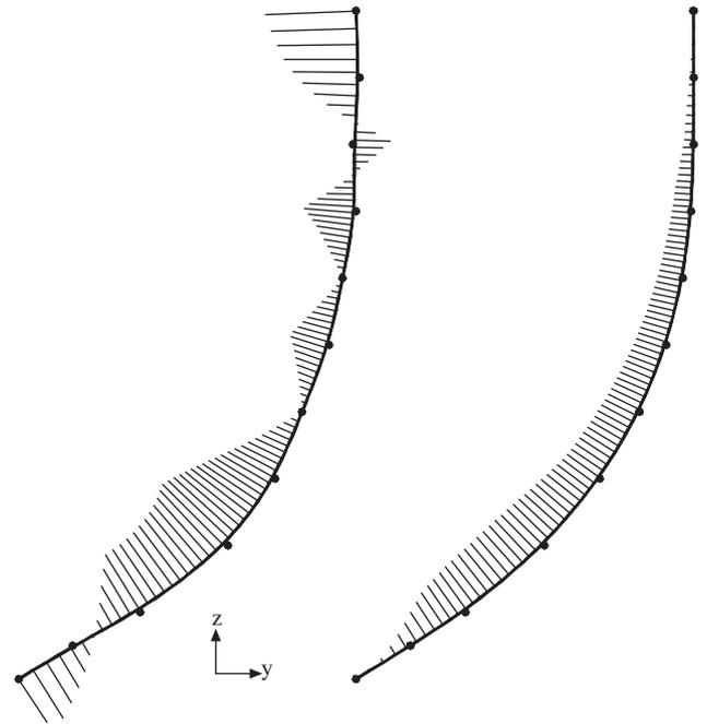
**Figure 4.** (a) Initial and (b) final V-shaped section (1050 iterations, 43% of improvement in the objective function).
