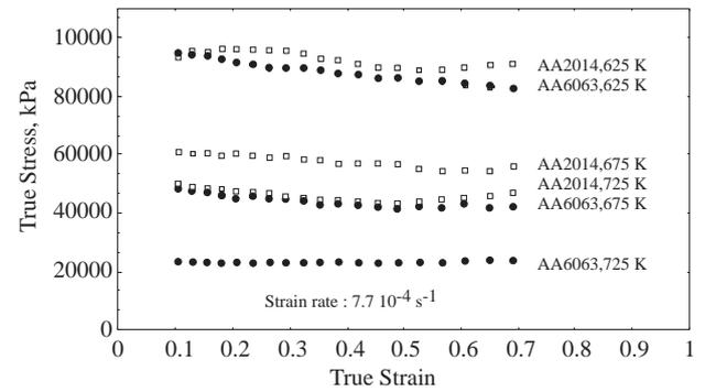
Figure 1. True stress-true strain curves.
