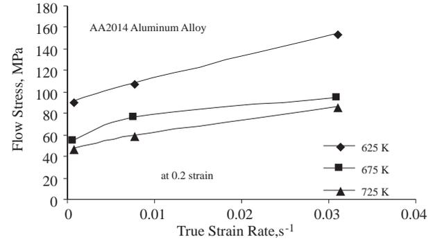
**Figure 2.** Changes in flow stresses with respect to temperatures and true strain rates
