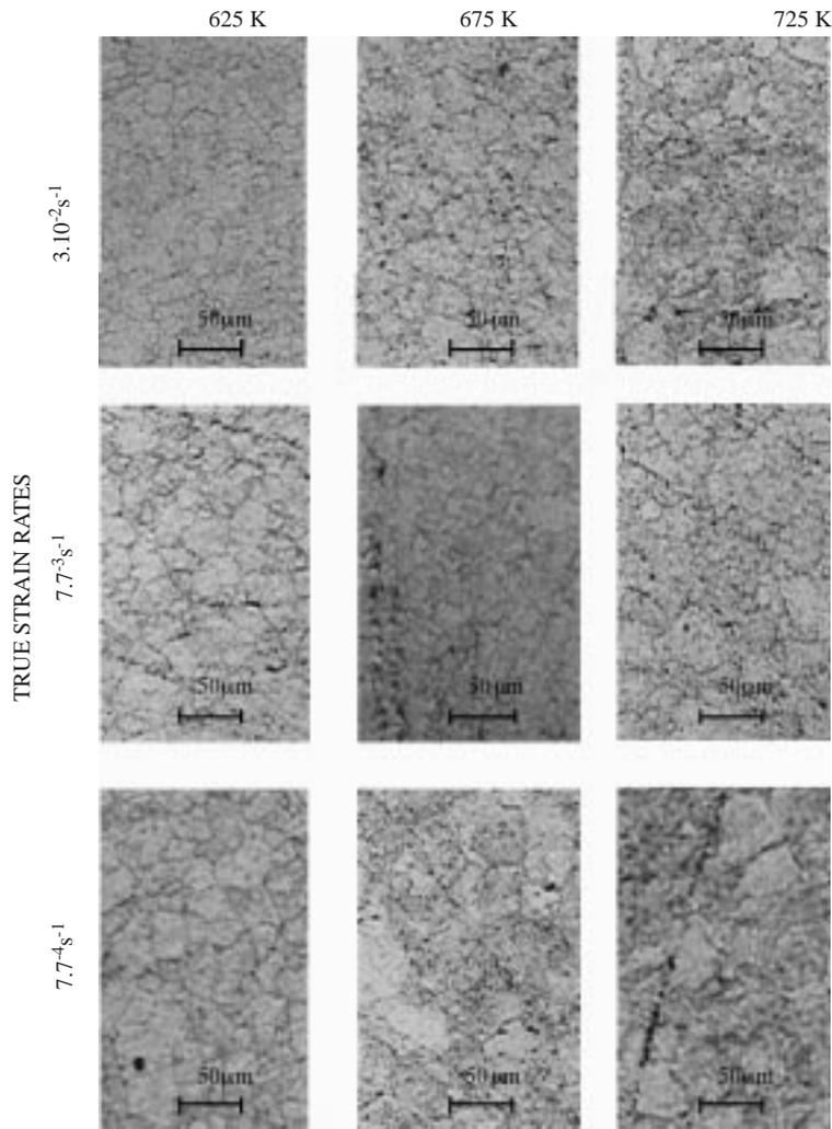
Figure 4. Micrographs of AA 6063 aluminum alloy after different tests.
