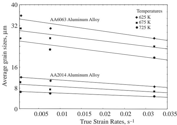
Figure 5. Functional changes in average grain sizes.
