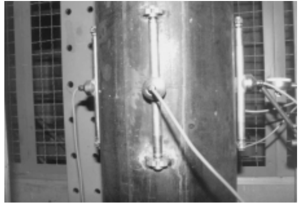
Figure 3. Installation of the dial gauges on steel tube
