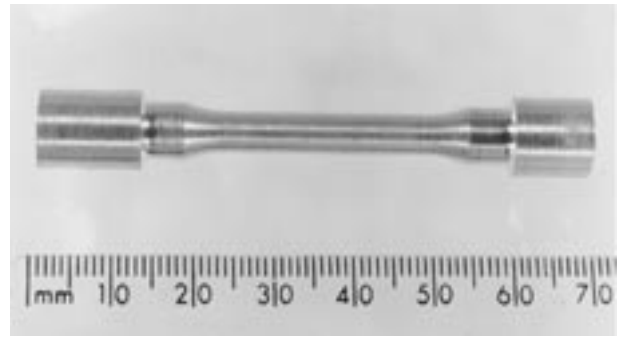
Figure 1. Photograph of a tensile test specimen used in this work (to BSEN 10002-1: 1990).
