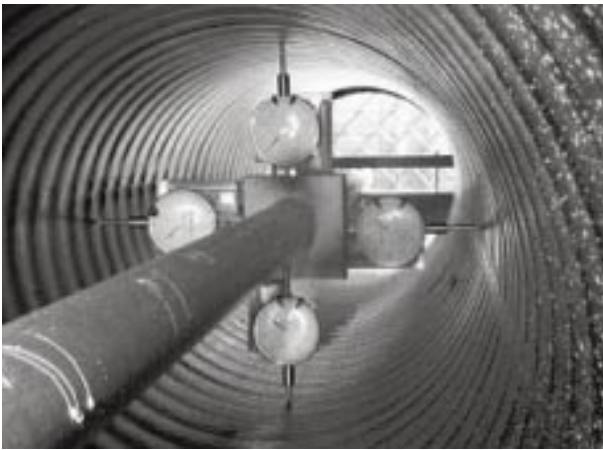
Figure 4. Set-up of dial gages
