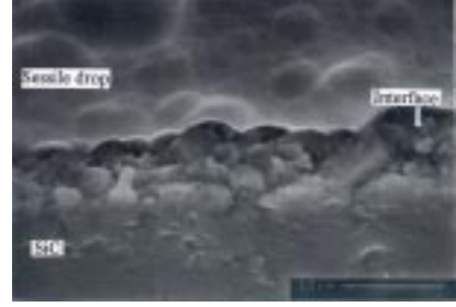
Figure 4. SEM micrograph showing the etched interface between Al-13.9Mg alloy sessile drop and sintered SiC (Etched in 2M NaOH).
