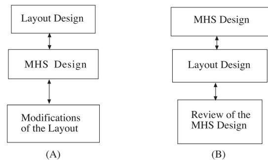
**Figure 1.** The Solution Sequence and Preferable Relations Between MHS and Facility Layout Design
