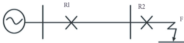
Figure 1. Primary and backup relay coordination in radial distribution system.
