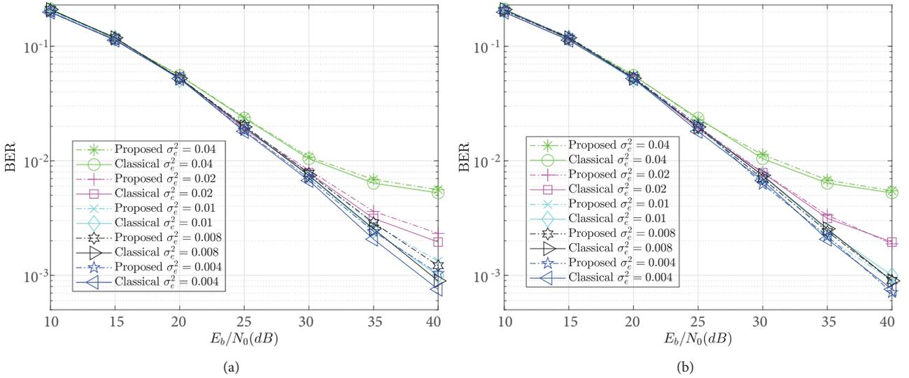
**Figure 4.** BER performances of the proposed scheme and conventional OFDM with 64-QAM and  $N = N_\alpha = 1024$  under imperfect channel estimation error (a) for Algorithm-2 (b) for Algorithm-1.
