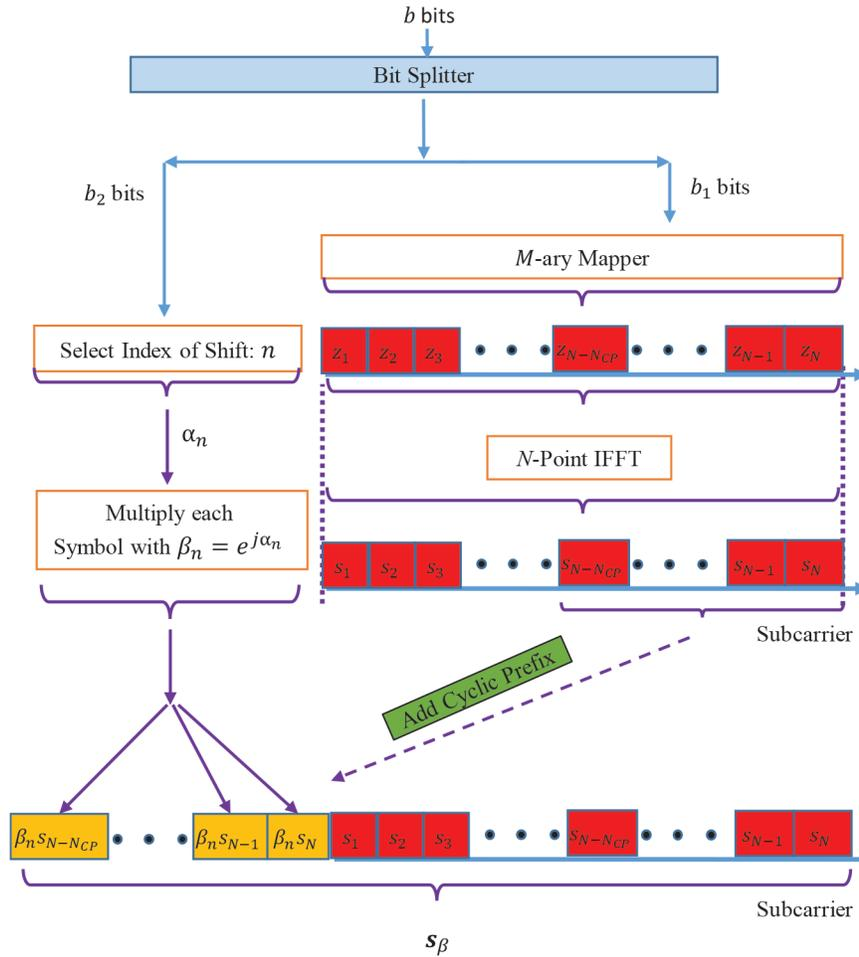
**Figure 1.** Frame structure of the proposed method.
