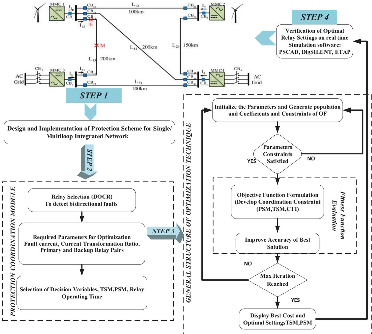
Figure 1. Protection strategy for integrated power networks.
