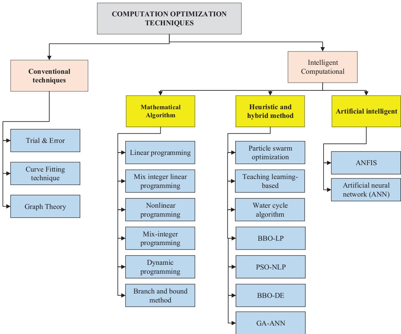
**Figure 2.** Optimal DOCR coordination with different optimization techniques.
