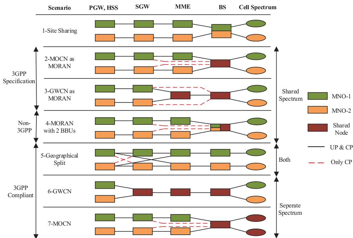
Figure 3. Different configuration options for RAN Sharing.
