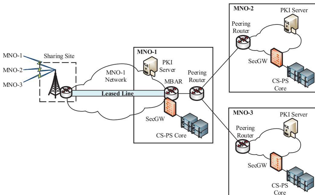
**Figure 4.** Topology of the target transport network.
