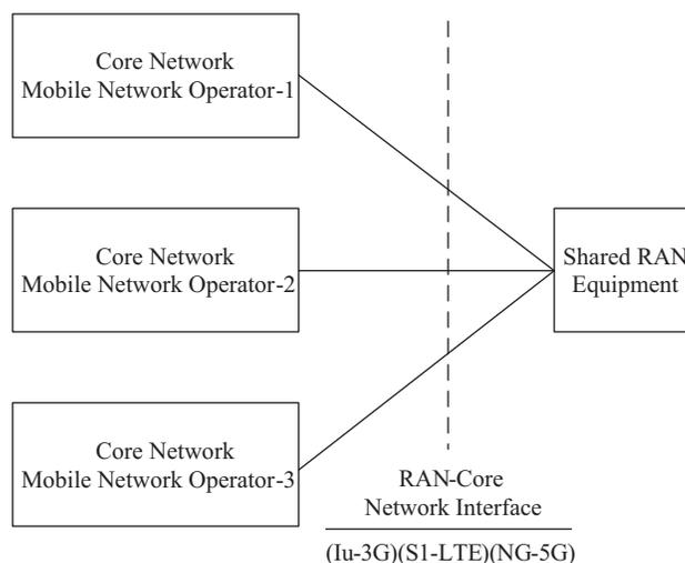
**Figure 1.** Multioperator-core-network-based RAN sharing scenario.
