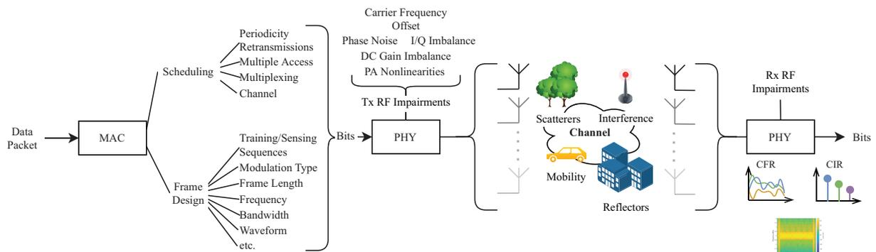
**Figure 1.** Illustration of the effects added to the signal as it traverses the environment.
