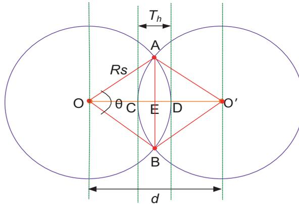
Figure 3. Two overlapping sensor nodes for full coverage.
