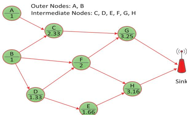
Figure 2. Illustration of load factor on sensor nodes.
