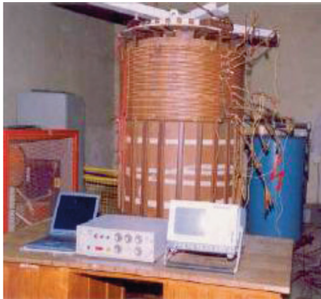
Figure 2. Experimental setup of a generator transformer.
