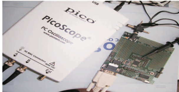
Figure 2. Experimental setup for FPAA-based implementation. AN221E04 type FPAA produced by Anadigm [1] has been used in this setup.
