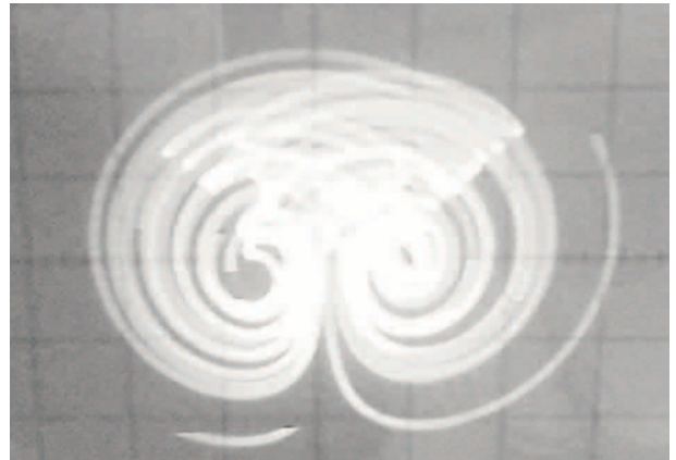
Figure 13. yz strange attractor as oscilloscope output of experimental circuit in Figure 10.
