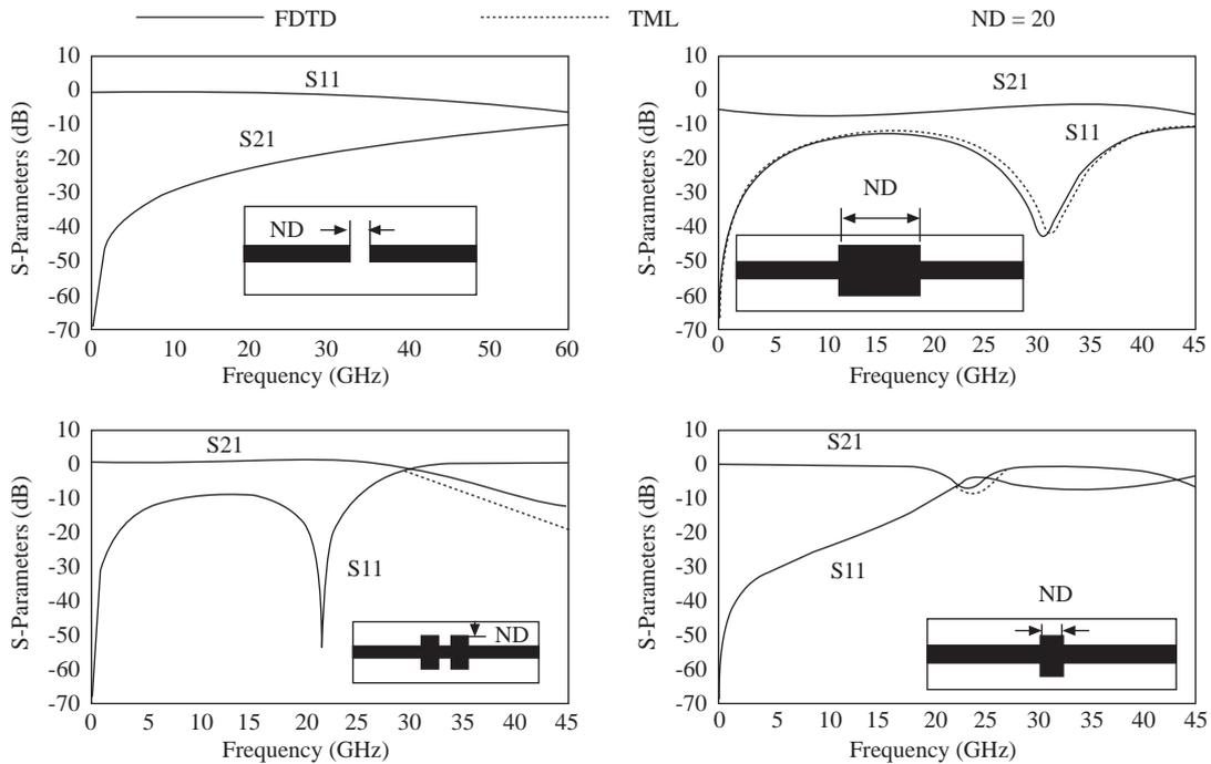
Figure 6. S parameters vs. frequency obtained via M-PATCH and TLM-ANT. (ND is the number of cells).
