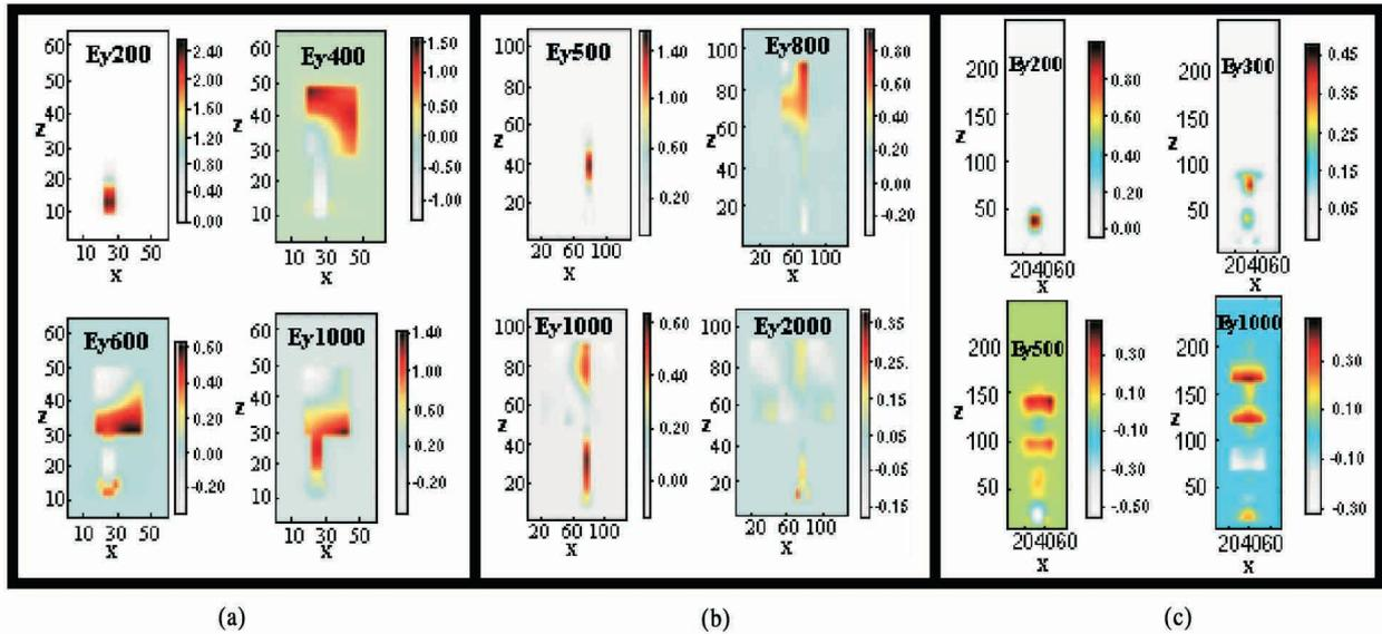
Figure 8.  $E_y$  on  $xz$ -plane, (a) line-fed rectangular patch, (b) 3-element coplanar patch (c) series-fed patch array.
