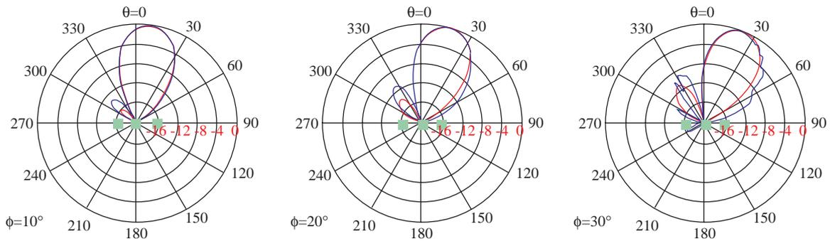
**Figure 13.** Beam forming with M-PATCH, 1.8 GHz, xz-plane, (solid: M-PATCH, dashed: M-PATCH plus analytical array factor formulation,  $\beta$ : beam steering direction).
