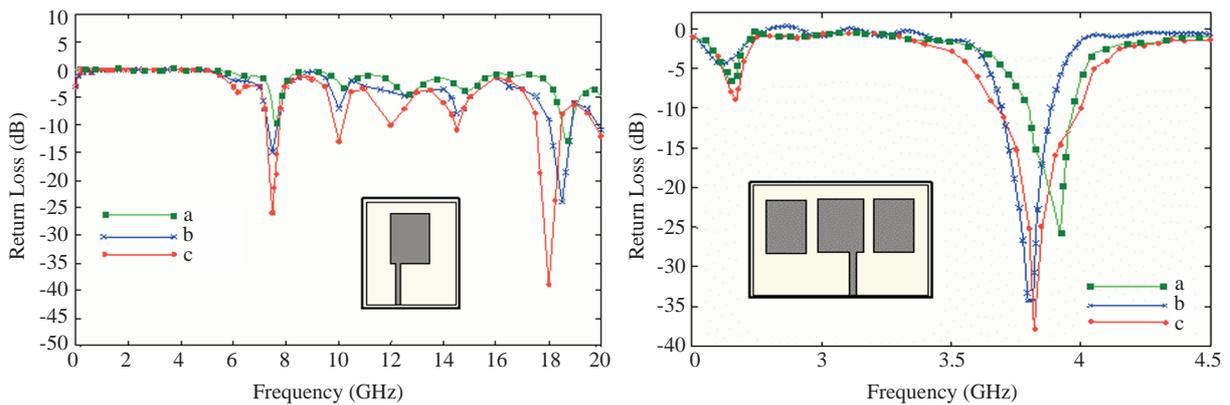
Figure 9. (Left) Return loss vs. frequency, (a) M-PATCH, (b) measurement [13], (c) FDTD [13]; (Right) Return loss vs. frequency, (a) FDTD [14], (b) M-PATCH, (c) measurement [14].
