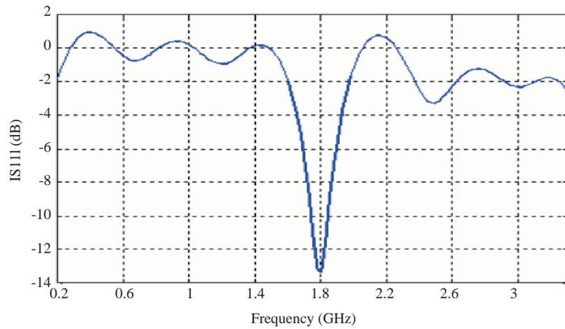
**Figure 11.** Return loss vs. frequency of a single patch ( $\Delta x = \Delta y = 2.76$  mm,  $\Delta z = 0.25$  mm,  $w = 20 \times \Delta$ ,  $a = 18 \times \Delta$ ,  $b_y = 5 \times \Delta$ ,  $b_x = 7 \times \Delta$ ).
