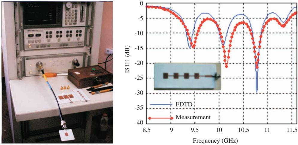
**Figure 10.** (Left) The measurement setup (HP 8510C Network Analyzer), (right) series-fed microstrip array, and return loss vs. frequency curves.
