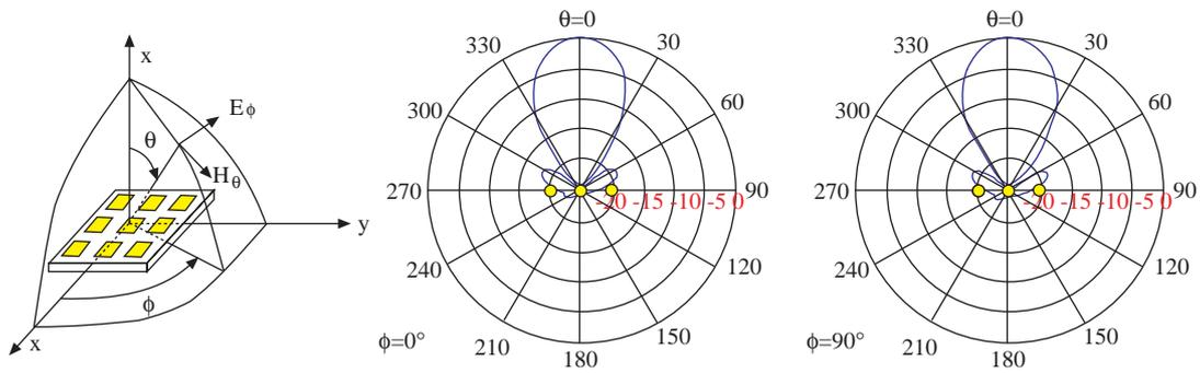
**Figure 12.** Radiation patterns at 1.8 GHz, left:  $\phi=0^\circ$ , right:  $\phi=90^\circ$ .
