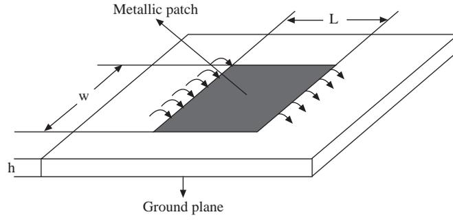
**Figure 1.** A rectangular patch antenna.
