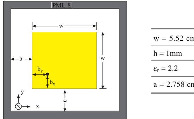
**Figure 2.** The square patch element and the dimensions.
