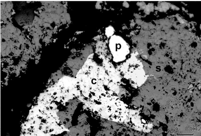
Figure 3. Photomicrograph of chalcopyrite partly replaced by sphalerite and pyrite (Binectaşı Mine), c: chalcopyrite, s: sphalerite, p: pyrite.
