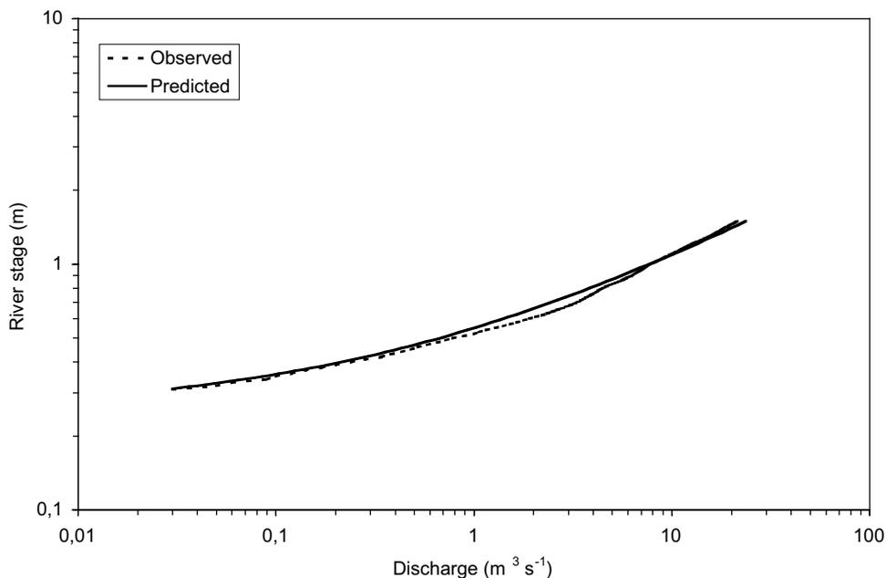
Figure 2. The stage-discharge rating curve for the Cwm Treweryn stream.
