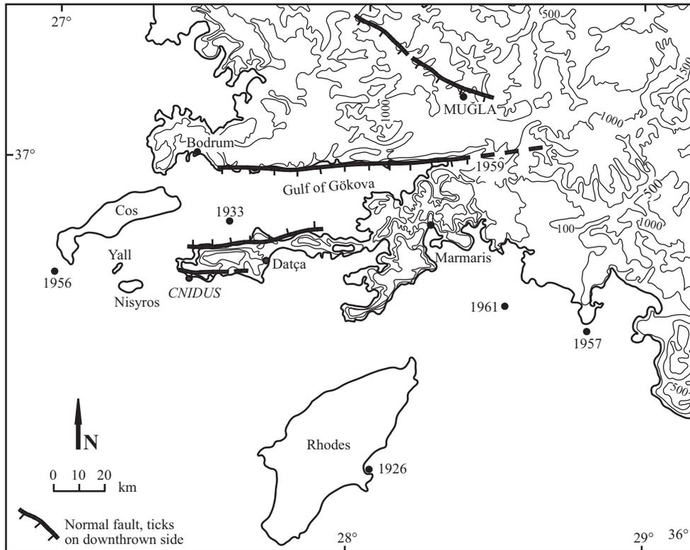
Figure 2. Structural and morphological setting of the Datça Peninsula. Bold lines show exposed active fault scarps in limestones, short lines on downthrown sides. Map also shows distribution of earthquakes with  $M \geq 6$  around Cnidus during the 20<sup>th</sup> century (Earthquake information taken from Ambraseys 1988 and McKenzie 1972).
