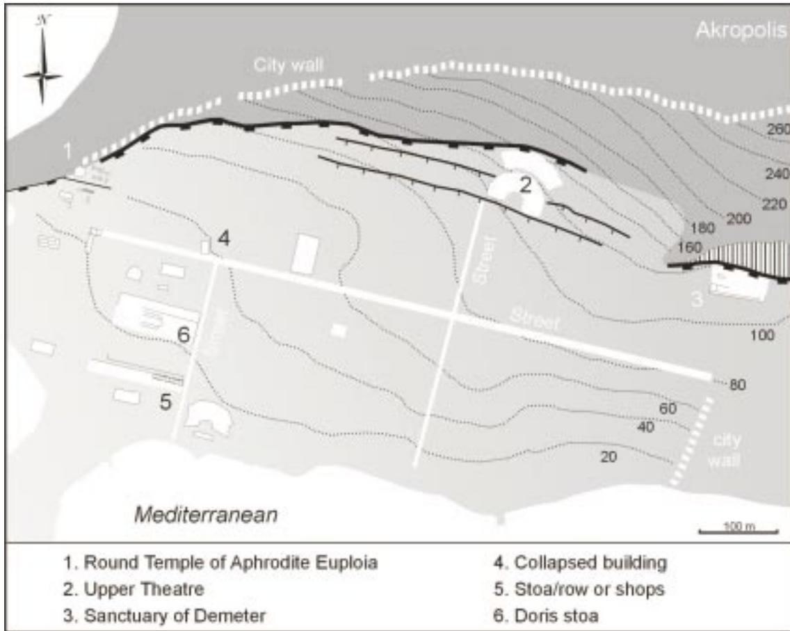
Figure 3. Plan view of key ruins at Cnidus. The bedrock limestone/Quaternary contact that marks the main trace of the Cnidus Fault is shown by the solid black line with boxes on the downthrown (south) side. Lines with bars indicate the trace of prominent morphological scarps cutting Quaternary scree deposits downslope of the bedrock fault scarp. Hashed ornament shows the decametre-high exhumed fault plane that forms the near-vertical back wall to the Sanctuary of Demeter.
