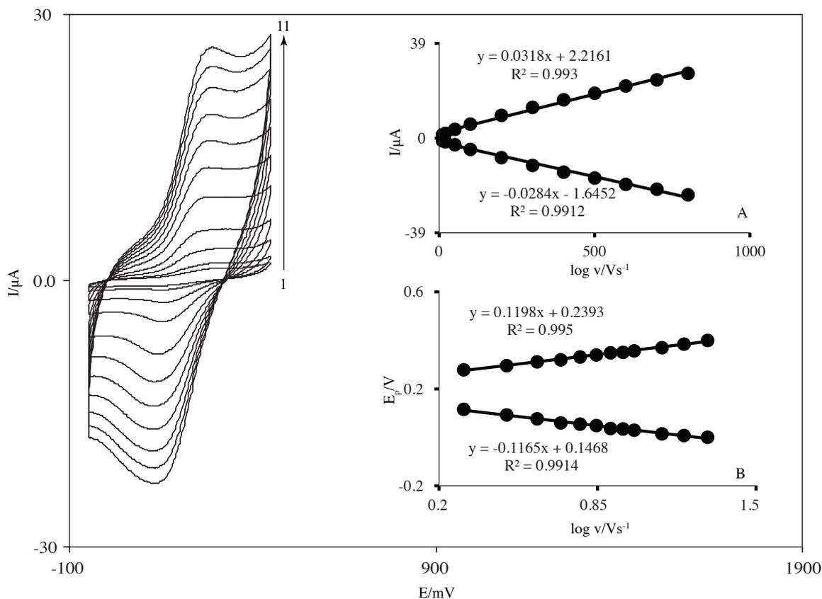
**Figure 1.** CVs of 5ADMBCNPE in 0.1 M PBS (pH 7.0), at various scan rates, numbers 1-11 correspond to 10, 20, 50, 100, 200, 300, 400, 500, 600, 700, and 800  $\text{mV s}^{-1}$ . Insets: variation of (A)  $I_p$  vs. scan rate; (B) Variation of  $E_p$  versus the logarithm of the high scan rates.
