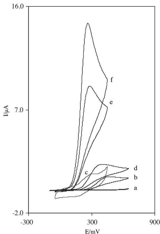
**Figure 2.** CVs of (a) unmodified CPE in 0.1 M PBS (pH 7.0), (b) unmodified CPE in 0.1 mM DA, (c) 5ADMBCNPE in 0.1 M PBS, (d) CNPE in 0.1 mM DA, (e) 5ADMBCPE in 0.1 mM DA, and (f) 5ADMBCNPE in 0.1 mM DA. In all cases the scan rate was  $10 \text{ mV s}^{-1}$ .
