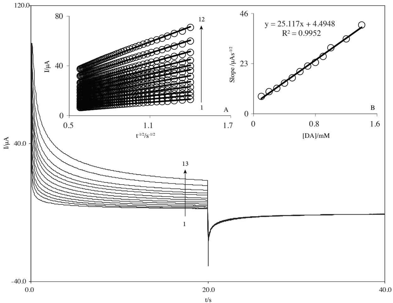
**Figure 4.** (A) Chronoamperograms obtained at 5ADMBCNPE in 0.1 M PBS (pH 7.0) for different concentration of DA. The numbers 1-13 correspond to 0.0, 0.1, 0.2, 0.3, 0.4, 0.5, 0.6, 0.7, 0.8, 0.9, 1.0, 1.2, and 1.4 mM of DA. Insets: (A) Plots of  $I$  vs.  $t^{-1/2}$  obtained from chronoamperograms 2-13. (B) Plot of the slope of the straight lines against DA concentration.
