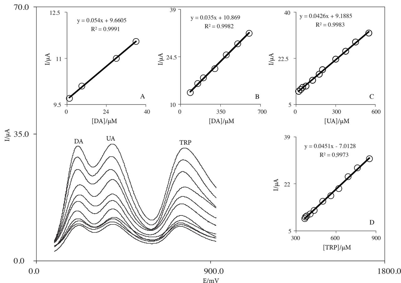
**Figure 5.** SWVs of 5ADMBCNPE in 0.1 M PBS (pH 7.0) containing different concentrations of DA + UA + TRP in μM, from inner to outer: 1.2 + 20.0 + 365.0, 7.5 + 35.0 + 370.0, 25.0 + 50.0 + 380.0, 35.0 + 75.0 + 405.0, 85.0 + 125.0 + 435.0, 150.0 + 175.0 + 500.0, 200.0 + 200.0 + 560.0, 300.0 + 300.0 + 620.0, 400.0 + 375.0 + 690.0, 500.0 + 450.0 + 760.0, and 600.0 + 550.0 + 850.0, respectively. Insets (A), (B), (C) and (D) are plots of  $I_p$  vs. DA, UA, and TRP concentrations, respectively.
