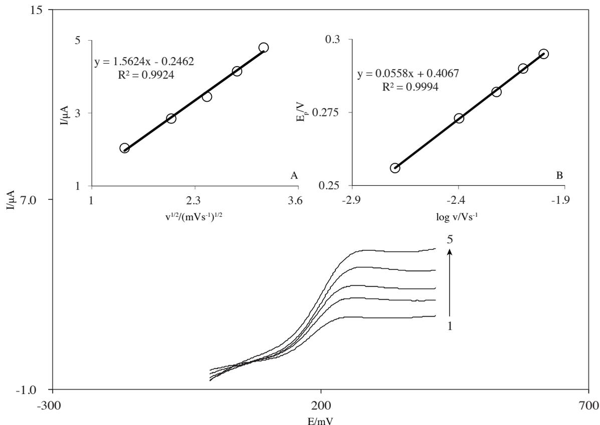
**Figure 3.** Linear sweep voltammograms of 5ADMBCNPE in 0.1 M PBS (pH 7.0) containing  $10.0 \mu\text{M}$  DA at various scan rates; numbers 1-5 correspond to 2, 4, 6, 8, and  $10 \text{ mV s}^{-1}$ , respectively. Insets: Variation of (A) anodic peak current vs.  $v^{1/2}$ ; (B) anodic peak potential vs.  $\log v$ .
