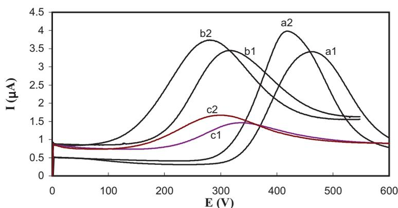
**Figure 6.** Differential pulse voltammograms for ANMGC (a1, b1, c1) and bare GC (a2, b2, c2) electrodes in PBS in the presence of 1.0 mM of mefenamic acid (a), 1.0 mM of indomethacin (b), and 1.0 mM of diclofenac (c).
