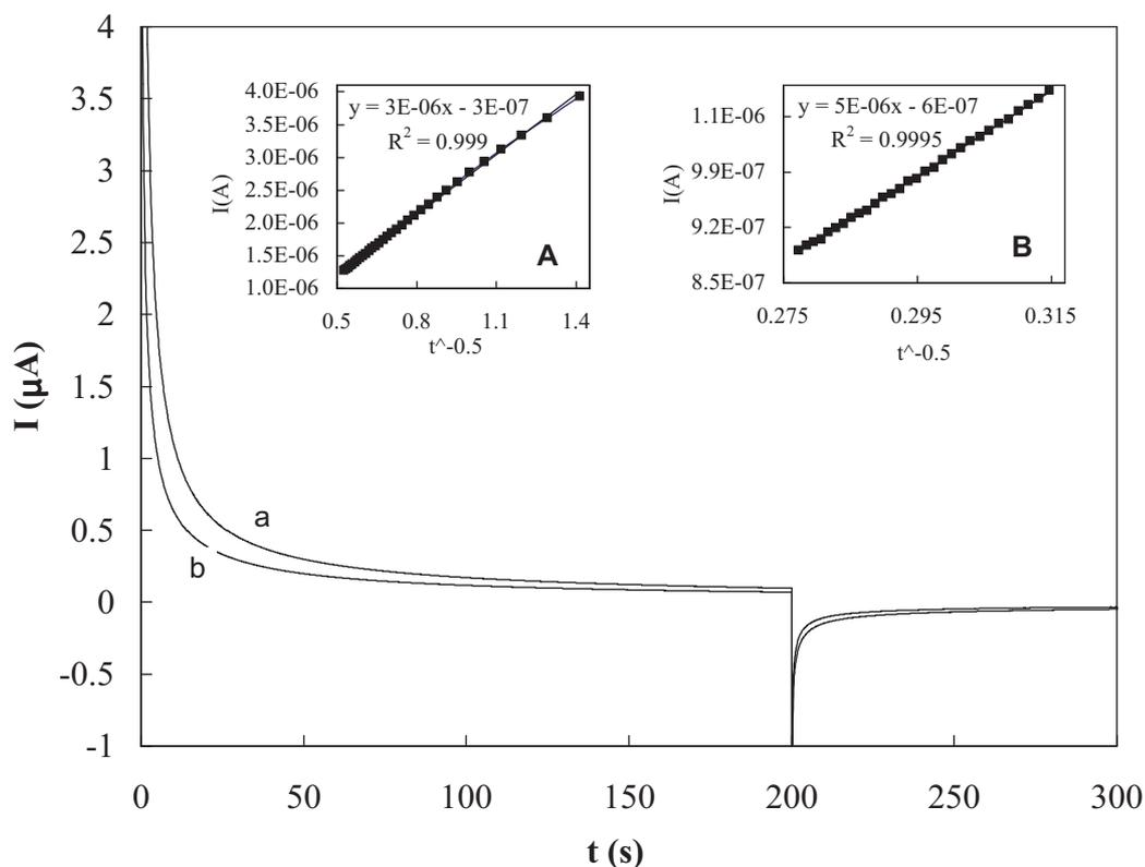
**Figure 4.** Double-step chronoamperograms of the GC (b) and ANMGC electrodes (a) in PBS solution containing 1.0 mM of mefenamic acid. Inset A: Dependency of the transient current on  $t^{-0.5}$  for the GC electrode. Inset B: Dependency of the transient current on  $t^{-0.5}$  for the ANMGC electrode.
