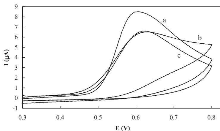
**Figure 3.** Cyclic voltammograms of the ANMGC electrode in the presence of 1.0 mM mefenamic acid (a), 1.0 mM indomethacin (b), and 1.0 mM diclofenac (c) in PBS. The potential sweep rate was  $50 \text{ mV s}^{-1}$ .
