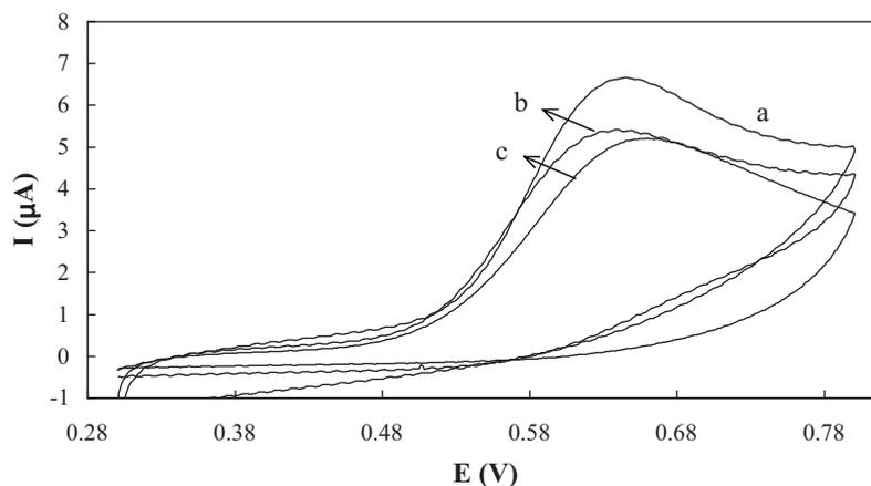
**Figure 2.** Cyclic voltammograms of the GC electrode in the presence of 1.0 mM mefenamic acid (a), 1.0 mM indomethacin (b), and 1.0 mM diclofenac (c) in PBS. The potential sweep rate was  $50 \text{ mV s}^{-1}$ .
