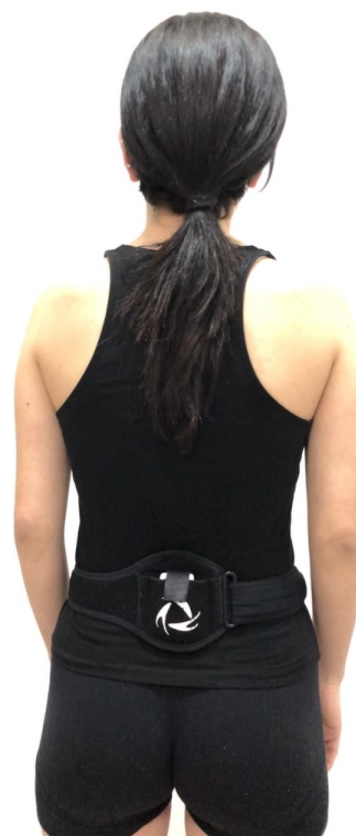
Figure 1. The G-Walk is placed on an elastic belt and worn on the waist.
