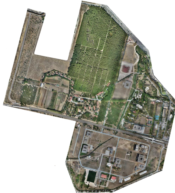
Figure 3. Produced approximately 2.5 cm orthomosaic of GTU campus area.
