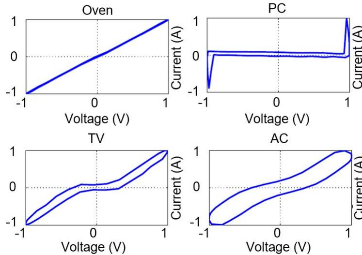
**Figure 6.** Examples of  $V$ - $I$  trajectory [59].
