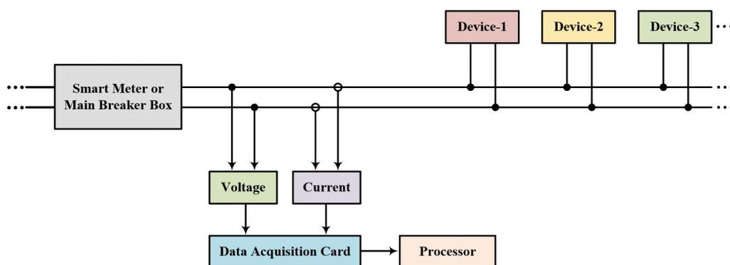
**Figure 2.** Acquisition of the aggregated power signal.
