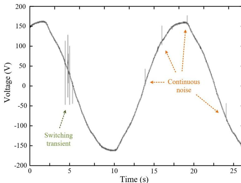
**Figure 8.** Voltage switching transient for blender [43].
