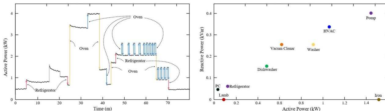
**Figure 5.** (a) Active power [15], (b) real-reactive power distribution [14].
