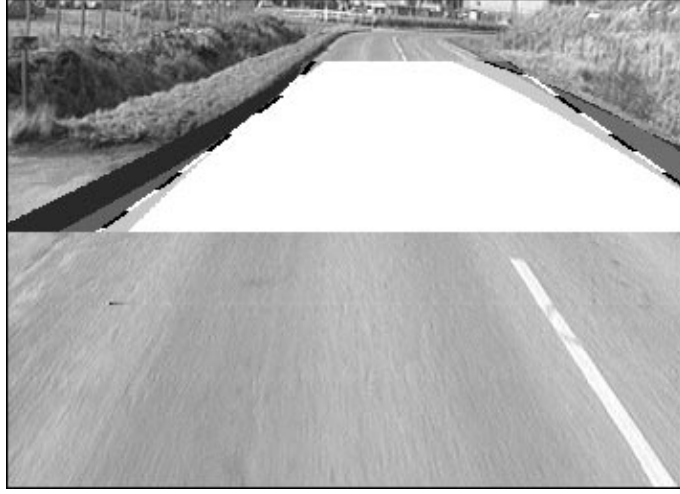
Figure 2. Pixel Voting Result. The different grey levels within the voting band of the Pixel-Based Fusion show the strength of belief that that a pixel is in the road. The final road edges displayed on the image are obtained by thresholding the voting space.
