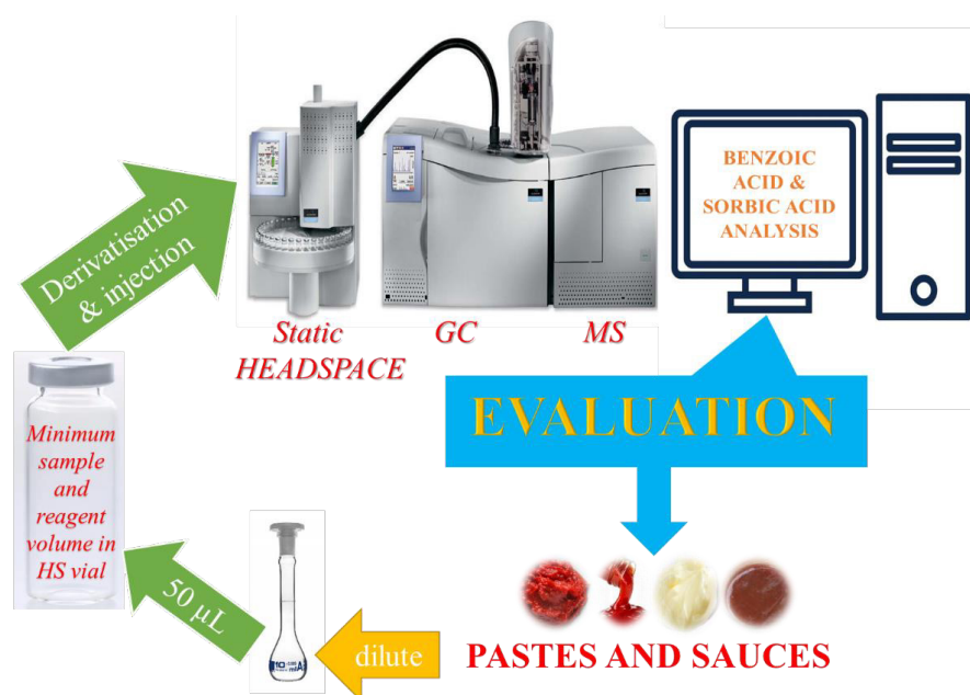
Figure 1. Graphical representation of simultaneous determination of BA and SoA in the pastes and sauces by using static HS-GC-MS.
