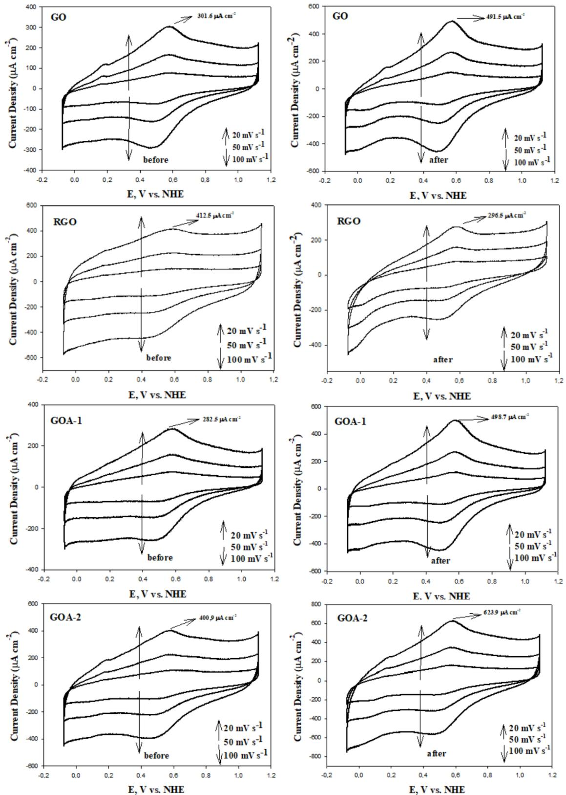
Figure 8. Cyclic voltammograms before and after carbon corrosion of graphene-based materials and graphene aerogels (potential range:  $-0.28$  to  $0.92$  V; scan rate: 20, 50, 100  $\text{mV s}^{-1}$ ; electrolyte:  $\text{N}_2$  saturated 0.1 M  $\text{HClO}_4$  solution).
