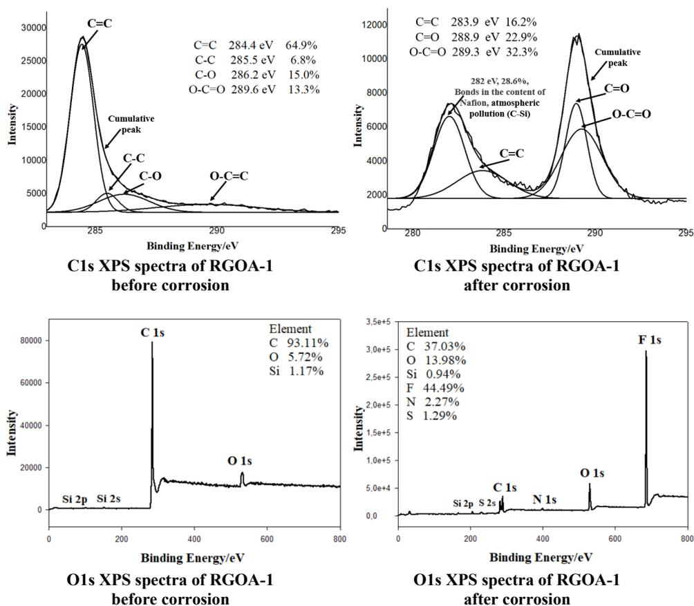
**Figure 12.** XPS spectra of RGOA-1 before and after corrosion.
