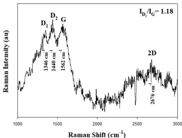
Figure 13. Micro-RAMAN spectra of RGOA-1 after corrosion.
