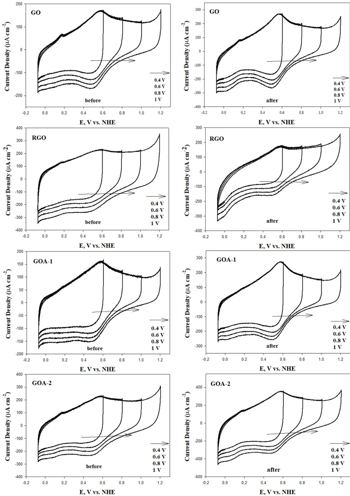
**Figure 9.** Cyclic voltammograms before and after carbon corrosion of graphene-based materials and graphene aerogels (potential range:  $-0.28$  to  $0.4$  V,  $-0.28$  to  $0.6$  V,  $-0.28$  to  $0.8$  V,  $-0.28$  to  $1$  V; scan rate:  $50 \text{ mV s}^{-1}$ ; electrolyte:  $\text{N}_2$  saturated  $0.1 \text{ M HClO}_4$  solution).
