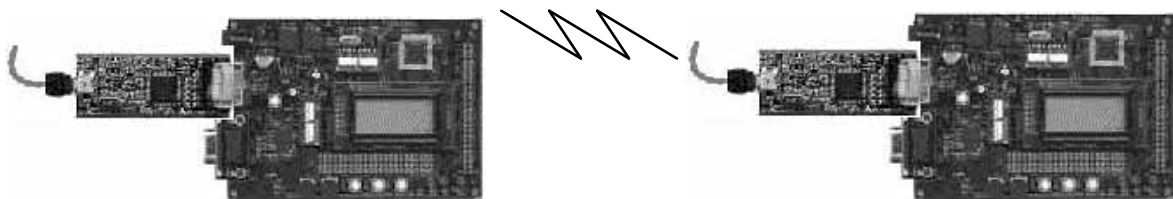
Figure 4. Sample embedded development board with proposed attached IEEE 802.15.4 communications daughter board.
