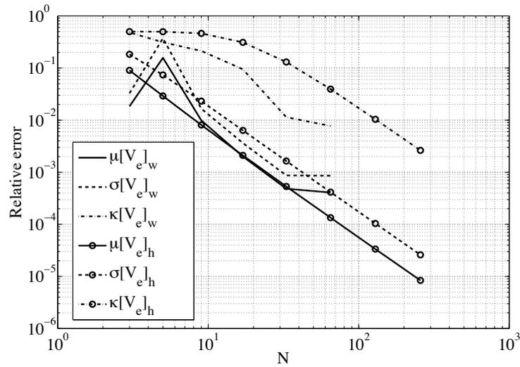
**Figure 4.** Relative error of the quadrature approximations of  $\mu[V_e]$  (solid lines),  $\sigma[V_e]$  (dashed lines) and  $\kappa[V_e]$  (dash-dotted lines) at  $f = 300$  MHz: wires  $S_w$  and  $S_h$  (circles).
