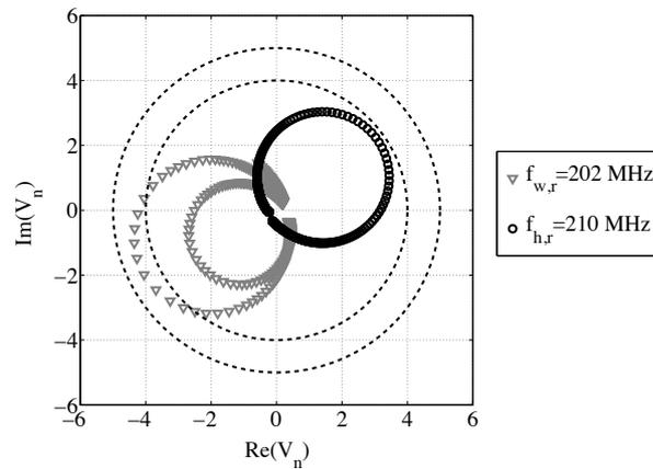
**Figure 10.** 1000 normalized samples  $V_n$  at resonances:  $f_{w,r}=202$  MHz for  $S_w$  and  $f_{h,r}=210$  MHz for  $S_h$ . Chebychev circles  $C_4$  and  $C_5$  (dashed lines).
