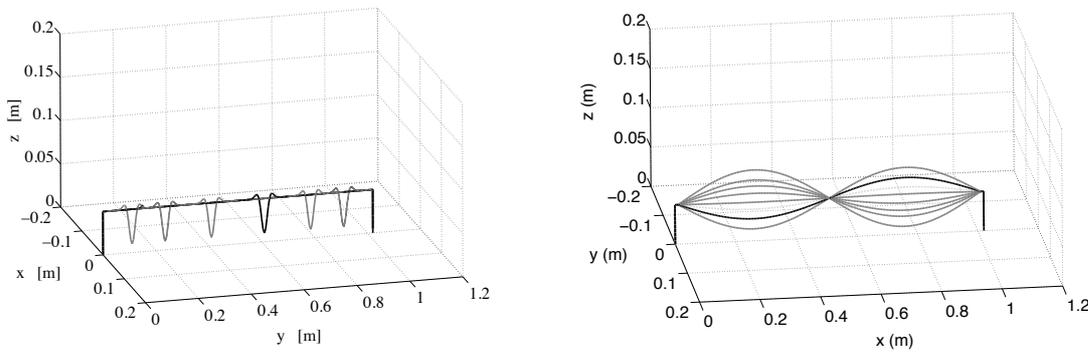
**Figure 2.** Examples of geometries resulting from the a local deformation (Figure (a)) and a global deformation (Figure (b)) of the axis of a thin wire.
