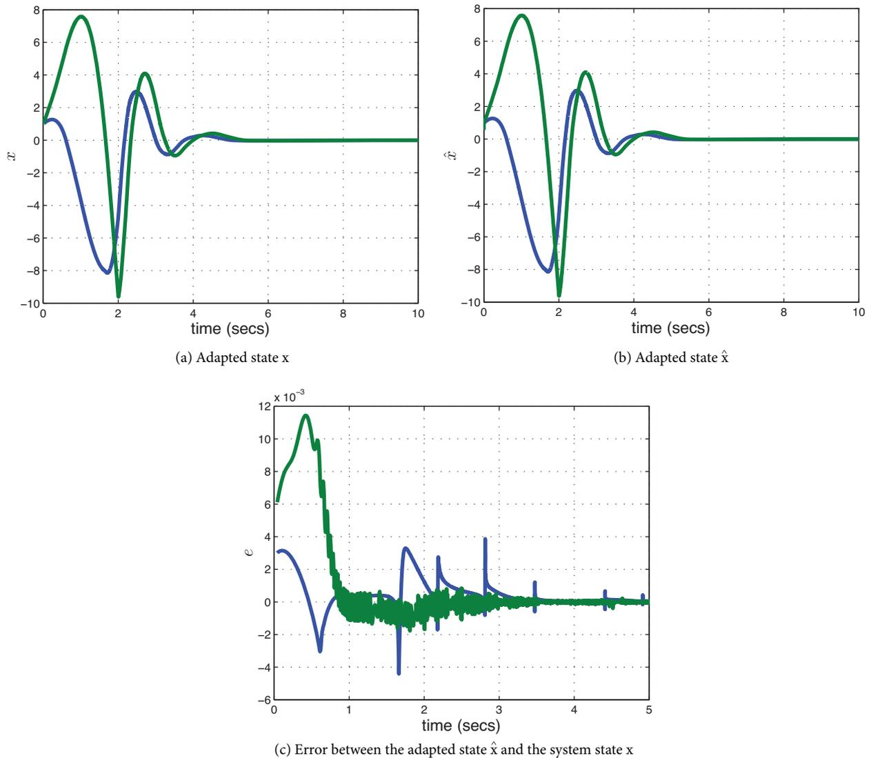
**Figure 6.** States of the flow system and adapted states with the controller turned on at  $t = 2$  seconds.
