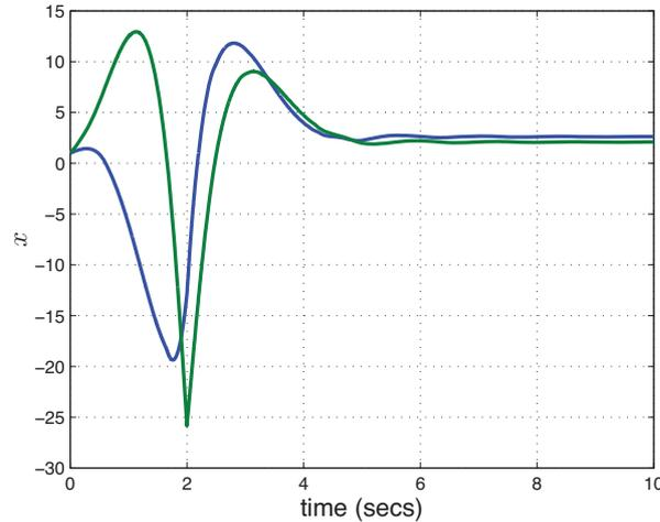
**Figure 8.** Response of the example system under LQR control, with the controller turned on at  $t = 2$  seconds.
