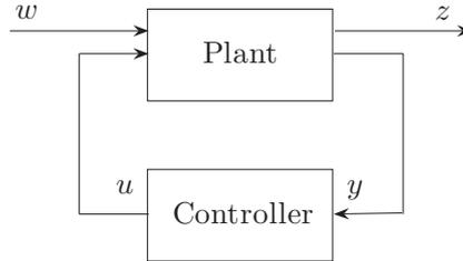
**Figure 2.** Feedback structure for linear parameter varying control design.
