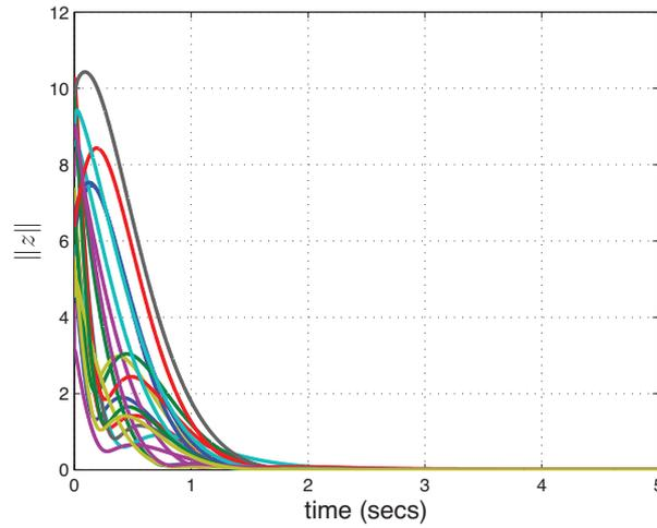
**Figure 5.** Response of the example system in closed-loop system for twenty random values of the parameter vector and initial conditions, under a step disturbance.
