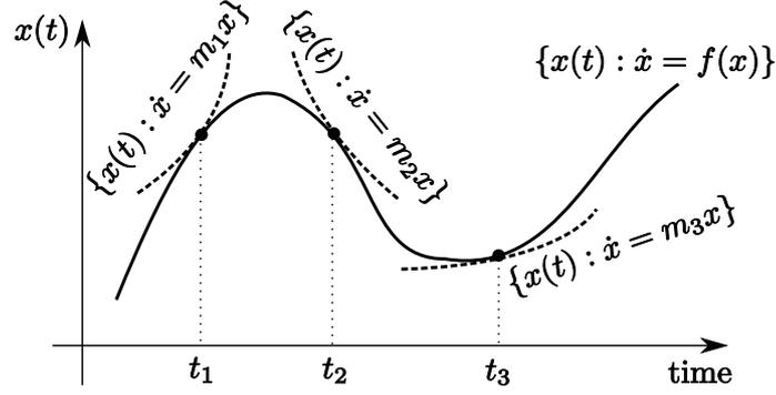
**Figure 1.** The motivation for approximating a nonlinear system with an LPV system.
