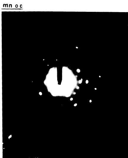
Figure 6. Diffraction pattern of 100:20 catalyst sample.
