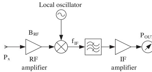
**Figure 1.** Block diagram of the total power radiometer.
