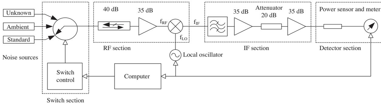
**Figure 2.** The configuration of the total power radiometer.
