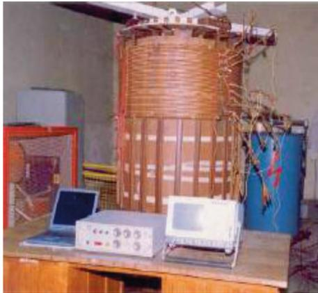
Figure 2. Experimental setup of a generator transformer.
