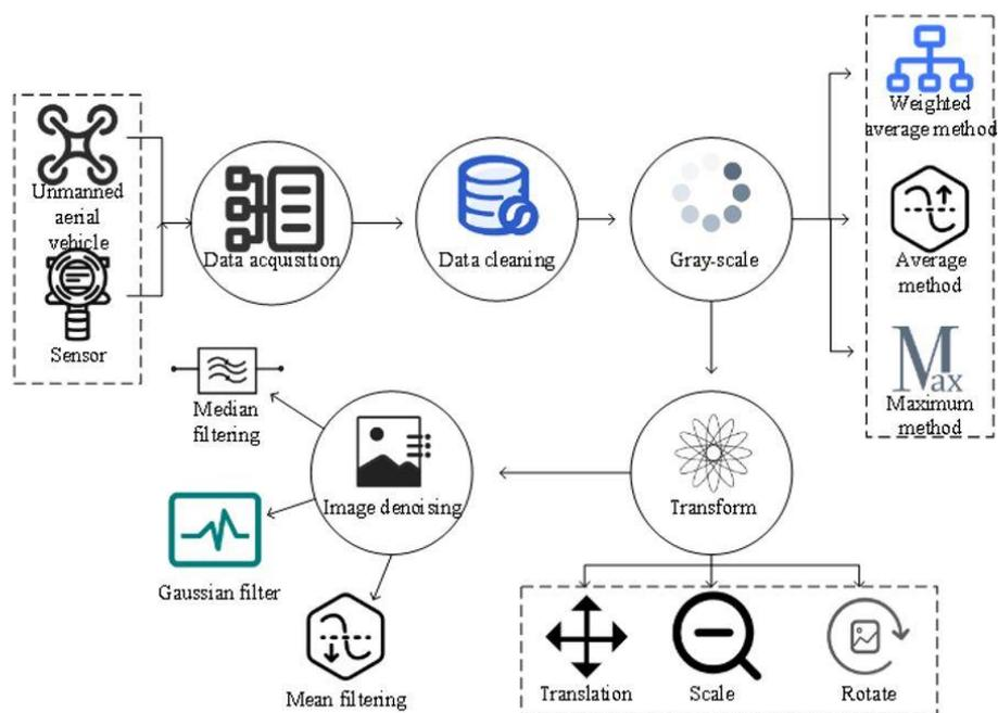
Figure 8. Operation flow structure of image data preprocessing.
