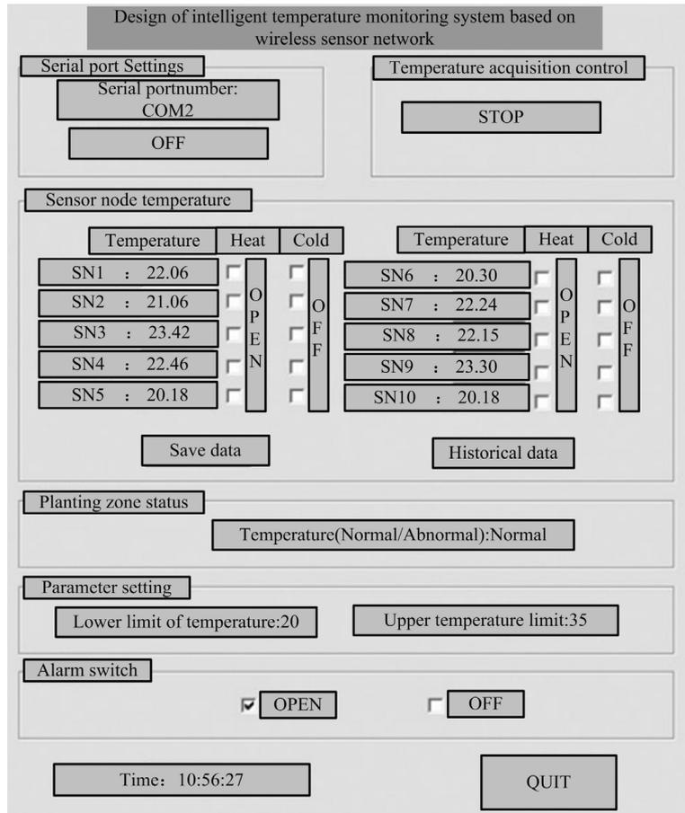
Figure 9. Display and control interface of the upper computer.
