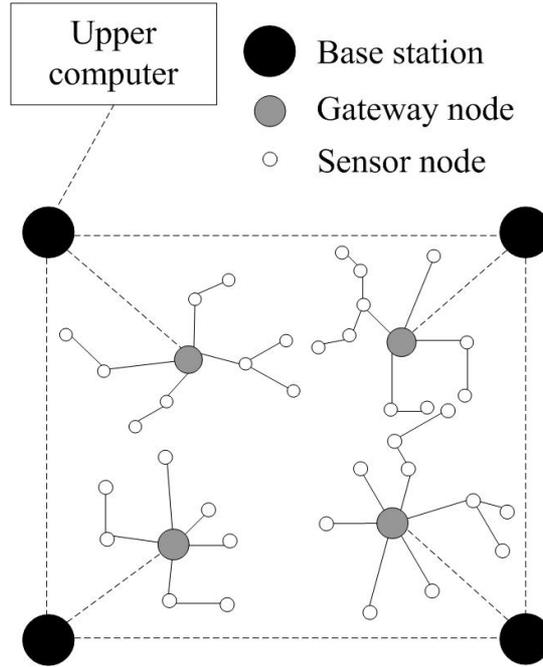
Figure 2. Architecture of the 3-layer WSN.
