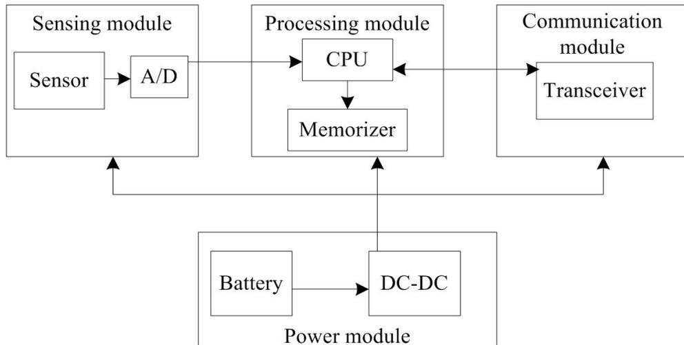
Figure 1. Wireless SN structure.
