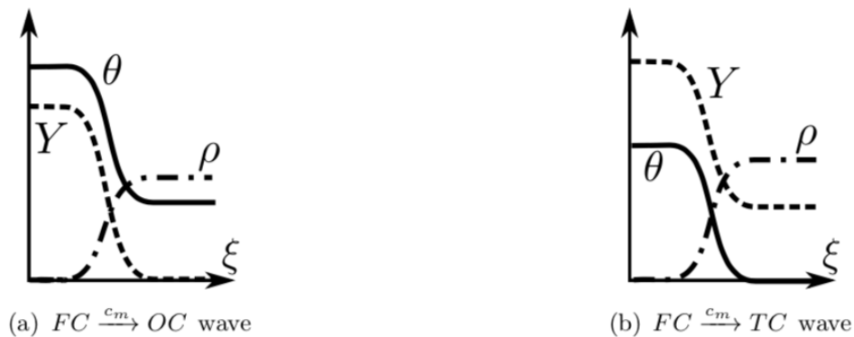
Figure 3. Intermediate combustion waves; \theta = temperature, \rho = solid fuel concentration, Y = oxygen concentration.
