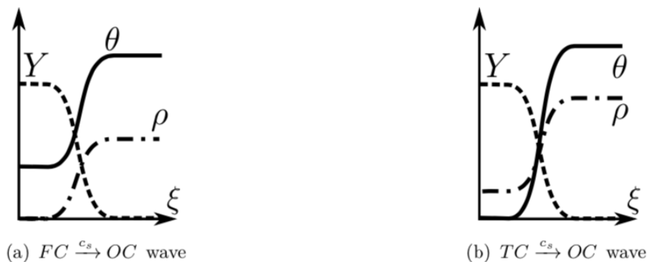
Figure 2. Slow combustion waves; \theta = temperature, \rho = solid fuel concentration, Y = oxygen concentration.
